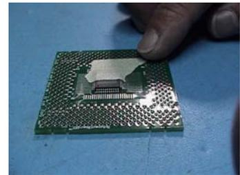
**3) Put Solder Flux along the base of the chip where it touches the board-**
